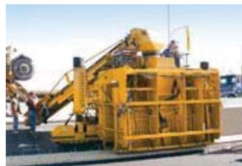
P.T. Ferro's barrier mold is built with double variable capabilities so each side of the wall can be adjusted for height.
